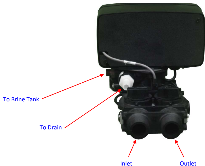
Fig 3: Fleck 5600 from the rear showing the inlet and outlet end-connector fittings 1" or 1-1/4" NPT in Noryl plastic. Brass end-connectors are also available for connecting to copper tubing.
